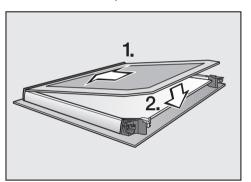
■ Push the inner pane into the plastic strip and place it between the retainers.
